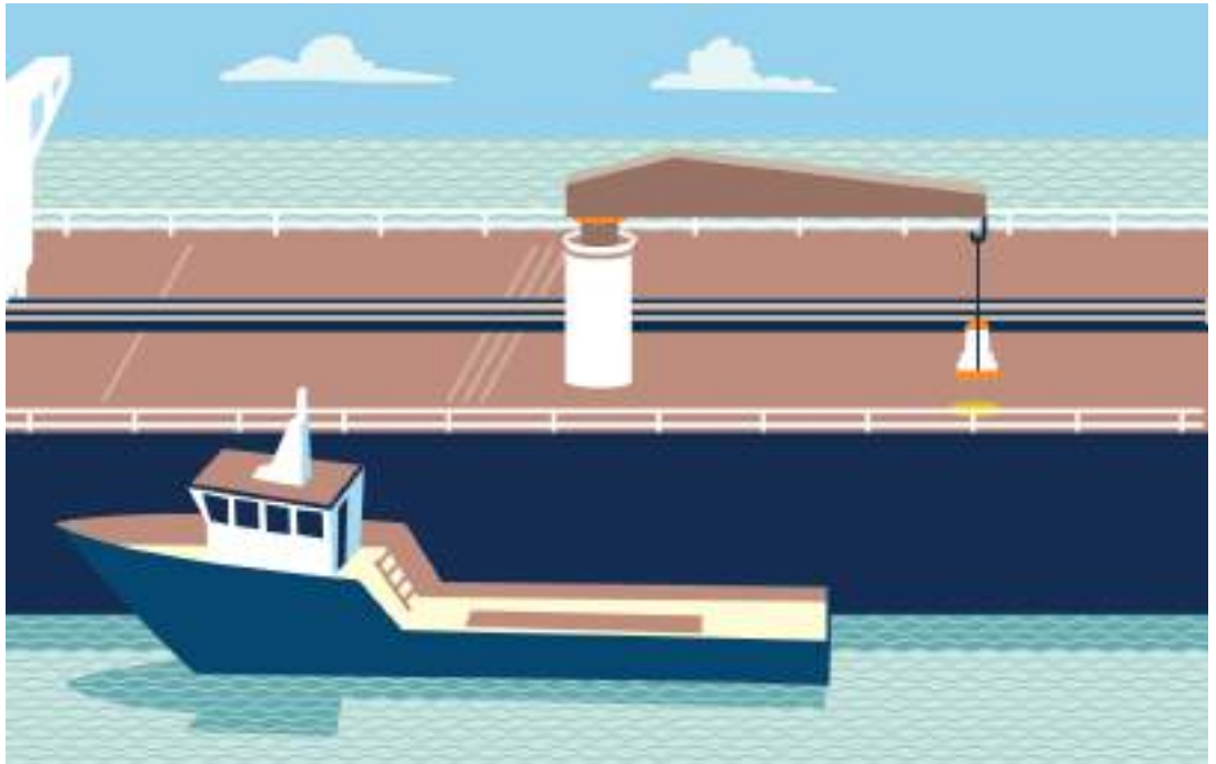
Figure 7.2: Personnel transfer by crane, bow to stern. The landing/lifting area in this situation should be forward of the manifold. This avoids interference with the support vessel's wheelhouse and masts.
