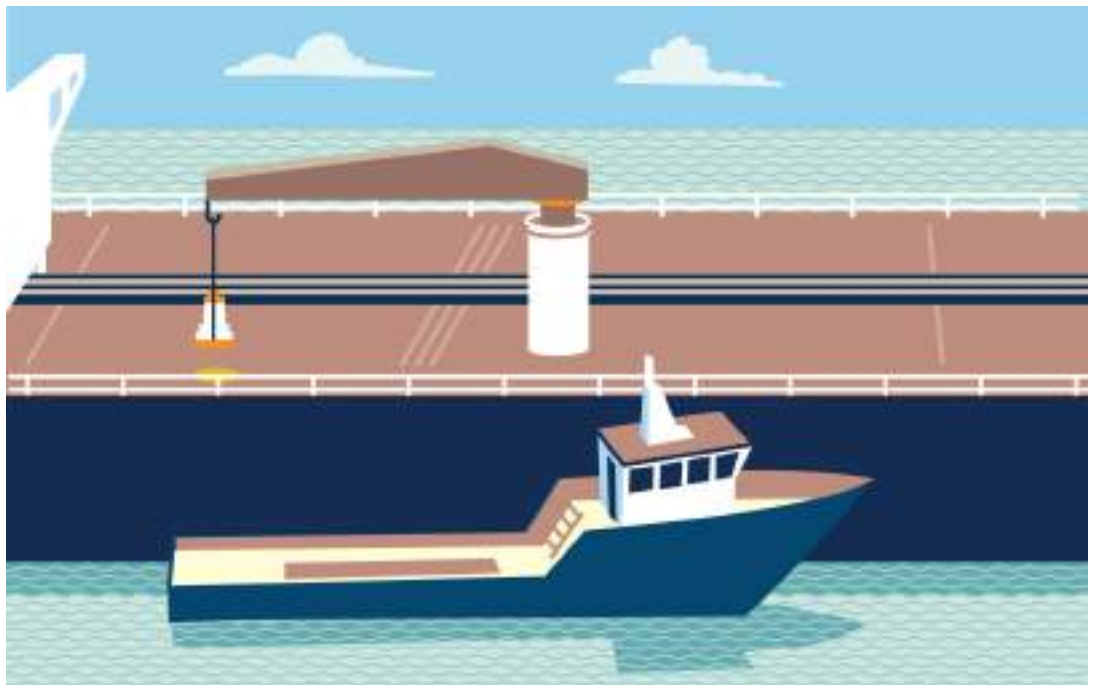
Figure 7.3: Personnel transfer by crane, bow to bow. The landing/lifting area in this situation should be aft of the manifold. This avoids interference with the support vessel's wheelhouse and masts.
